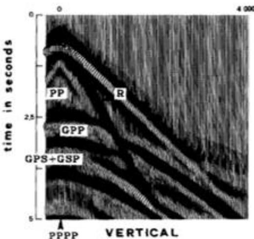
Fig. 3. Seismograms in which the various reflections can be observed in the upper part can be seen the horizontal
