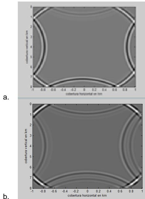
Fig. 4. Comparison of the application of the scheme of reduction of the reflection of the wave at the edges. Part a shows the modeling of the wave without the attenuation and in part b is the attenuation of the absorption of the edges.
